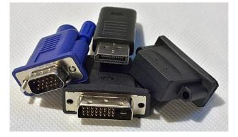
These cheap gadgets can also give you two monitors to remote into instead of one. Right, with dummy plugs, you can remote into a computer that's running in a closet with no cables but power and network, and still have multiple virtual screens available for your work, up to the limit of how many physical monitors are usable by both of the computers in use.
